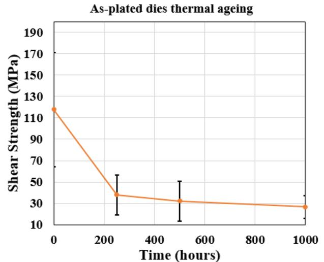
Figure 4. Shear strengths of assemblies with as-plated Cu bumps over isothermal ageing at  $200^{\circ}\text{C}$  – 1000hours
