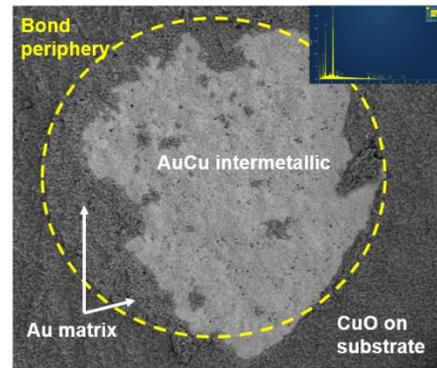
Figure 7. BSE-SEM of sheared substrate interface with planarized die aged isothermally at  $200^\circ\text{C} - 1000$ hours with SEM-EDX elemental chart as inset
