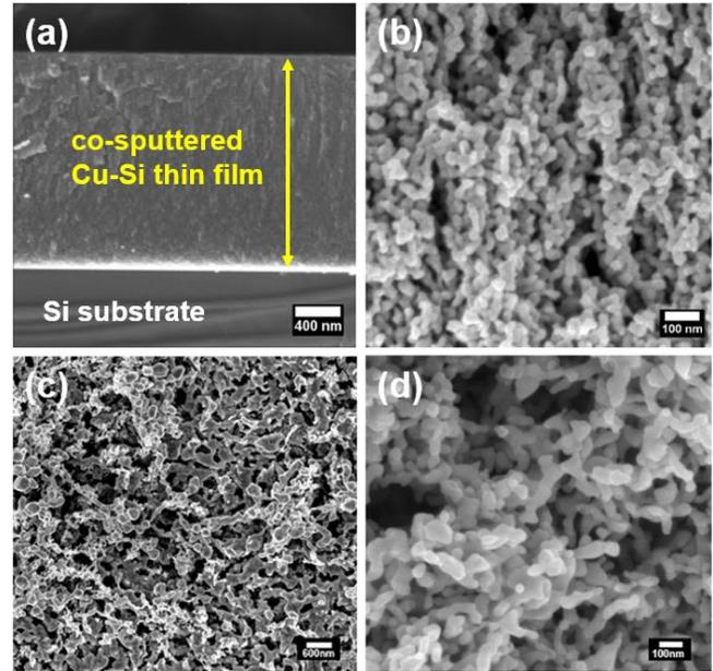
Figure 8. Cross-sectional SEM images of (a)-(b) co-sputtered Cu-Si thin film and dealloyed nano-Cu foam; plan-view SEM images of (c) macro-Cu foam and (d) nano-Cu foam from dealloyed Cu-Zn
