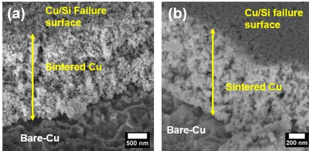
Figure 9. SEM cross-sectional view of fractured sintered nano-Cu joint on bare-Cu assembly at (a) 200°C and (b) 250°C
