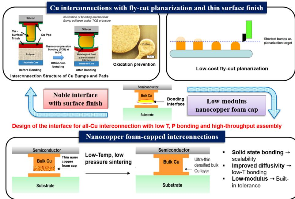
Figure 2. Unique GT – PRC approaches towards all-Cu interconnections without solders
