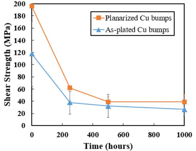
Figure 6. Comparative shear strengths of assemblies with as-plated and planarized Cu bumps over isothermal ageing at  $200^\circ\text{C} - 1000$ hours
