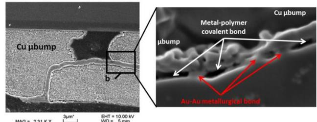
Figure 3. SEM cross-section of as-plated Cu bump-on-pad assembly with pre-applied underfill trapped in interfacial voids
