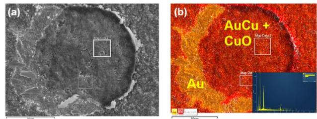
Figure 5. SEM-EDS of the sheared substrate interface aged isothermally at  $200^{\circ}\text{C}$  for 1000 hours
