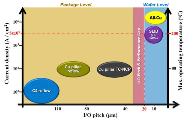
Figure 1. Metrics for off-chip interconnection pitch and performance scaling in advanced packaging
