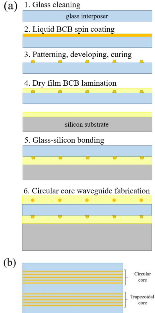
Figure 4. (a) Fabrication process of the complete sample and (b) schematic of the top view of a diced sample with waveguides of both cross sections.
