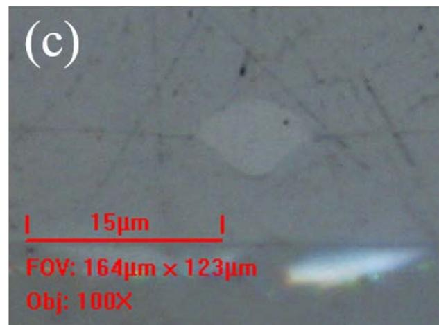
Figure 5. Cross section images of (a) a waveguide core with left-shift on top, (b) a waveguide core with right-shift on top, and (c) a waveguide core without shift.
