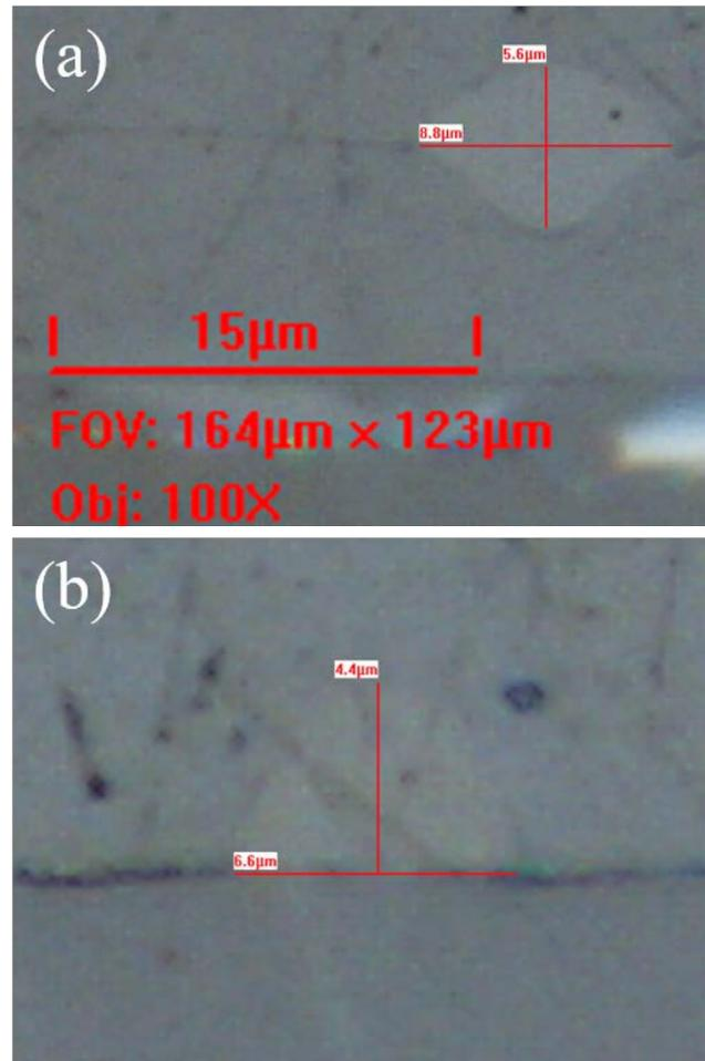
Figure 6. Height and width measurements: (a) Circular core and (b) trapezoidal core.
