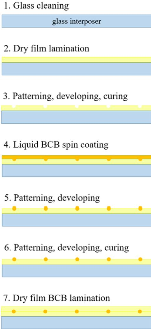
Figure 3. Fabrication of circular core waveguides.
