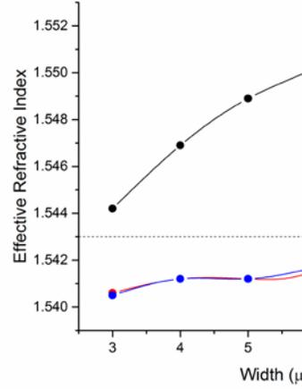
Figure 2. Mode simulation of trapezoidal waveguide with 6  $\mu\text{m}$  height by COMSOL beam-envelope method for 1.550  $\mu\text{m}$  wavelength.
