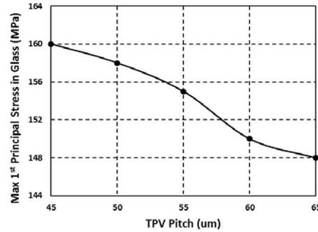
**Figure 8.** Change in maximum 1<sup>st</sup> principal stress in glass for varying TPV pitch.
