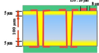
**Figure. 3** Stack up dimension of the test vehicle
