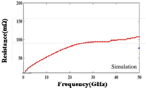
Figure.14 AC Resistance of a signal TPV
