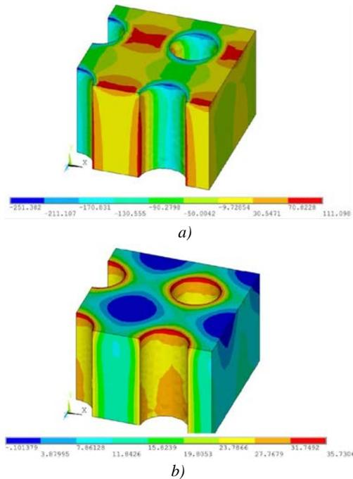
**Figure 7.** Contour plots of (a) stress in Cartesian direction ( $\sigma_{xx}$ ) (MPa) and (b) 1<sup>st</sup> principal stress (MPa) in glass for  $50\text{ }\mu\text{m}$  pitch.
