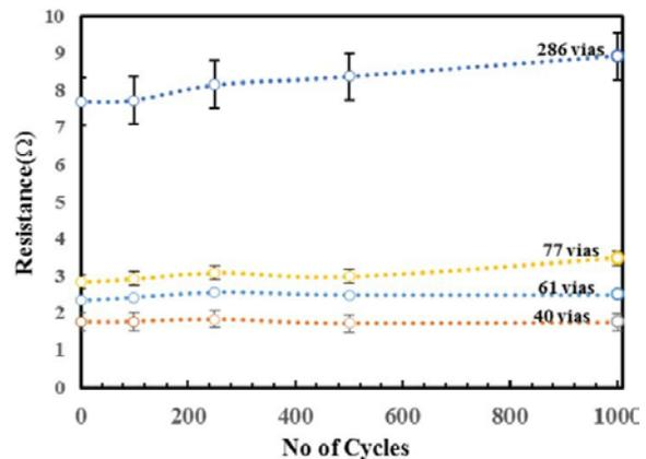
**Figure 9.** DC Resistance of TPV chains during TCT.
