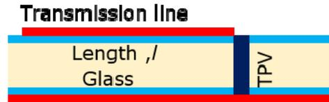
**Figure 13.** Input Impedance method for estimating TPV parasitics
