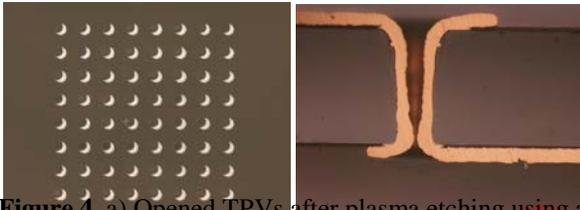
**Figure 4.** a) Opened TPVs after plasma etching using a copper etch mask. b) Cross section of metallized TPV
