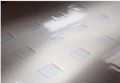
Figure 11. Top view of GFO package after polymer lamination
