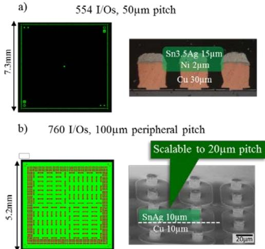
Figure 1. Test vehicle designs with a) standard Cu pillars, and b) ultra-short Cu pillars with reduced solder height.
