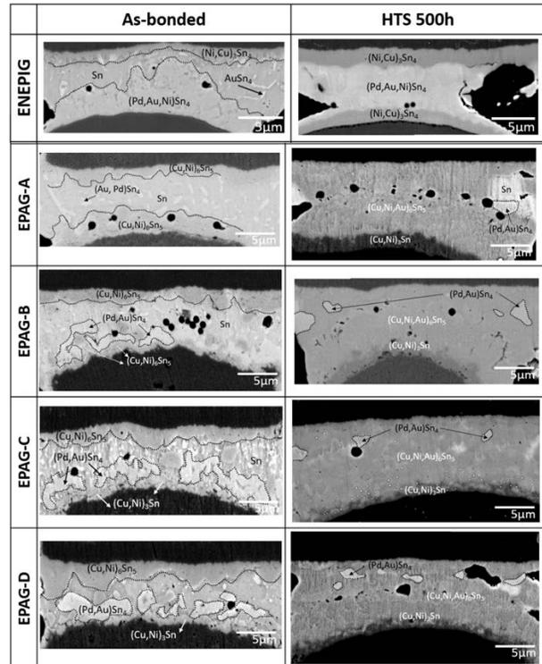
Figure 2. Interfacial characterization of assemblies with standard Cu pillars through 500h HTS at 150 $^{\circ}$ C.
