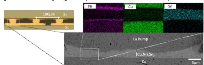
Figure 7. SEM/XEDS analysis of as-bonded metastable SLID joints.
