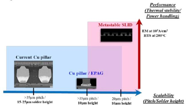
Figure 14. Georgia Tech PRC's roadmap to high-performance, ultra-fine pitch C2S solder-based interconnections.
