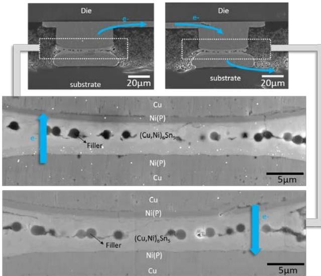
Figure 9. Metastable SLID joints after 1000h of current stressing at  $10^5 \text{ A/cm}^2$ , 150°C.
