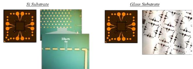
Figure 11. Silicon and glass substrates with metalization at 20µm I/O pitch.
