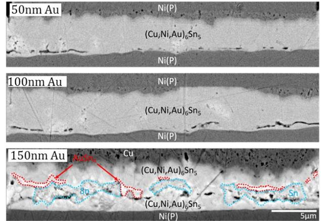
Figure 6. Microstructure of metastable SLID interconnections with varying Au thickness of ENIG surface finish.
