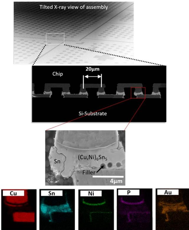
Figure 12. Metastable SLID bonding at 20µm pitch on Si substrate.
