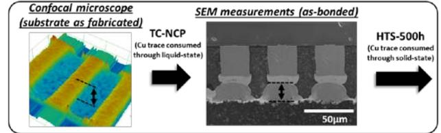
Figure 4. Method for quantification of Cu consumption from the substrate traces.
