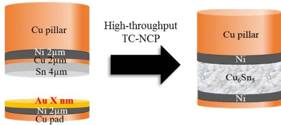
Figure 5. Metastable SLID bonding concept for applicability to chip-to-substrate interconnections.
