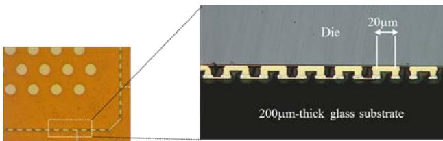
Figure 13. Metastable SLID bonding at 20µm pitch on glass substrate.
