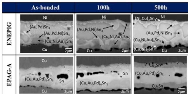
Figure 3. Interfacial characterization of assemblies with ultra-short Cu pillars without barrier layer through 500h HTS at  $150^{\circ}\text{C}$ .
