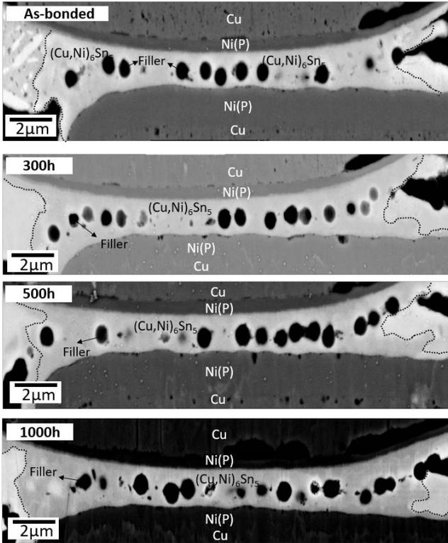
Figure 8. Microstructural evolution of metastable SLID joints through 1000h of HTS at 200°C.
