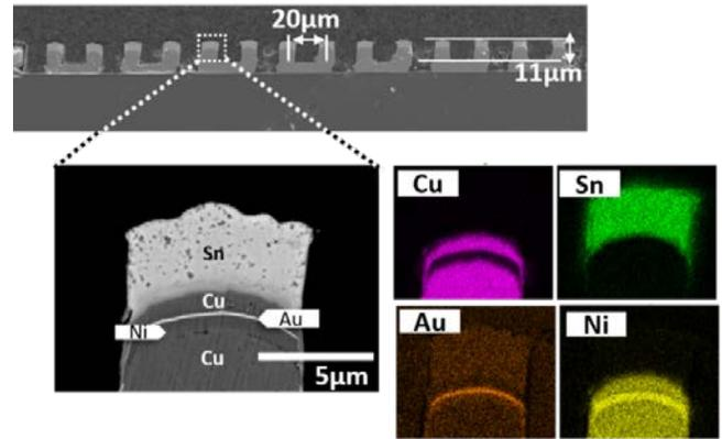
Figure 10. Bumped Si daisy-chain test die at 20µm pitch.
