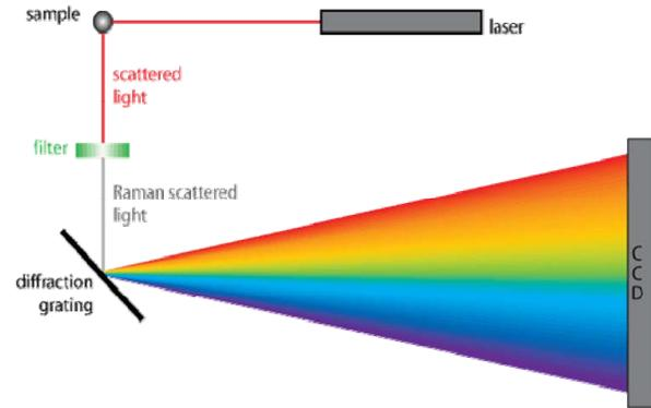
Figure 2. Raman spectrometer scheme
