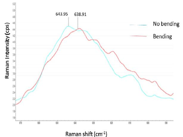
Figure 9. Raman Spectrum during bending of glass
