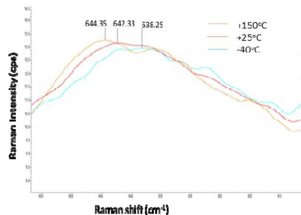
Figure 10. Raman spectrum during thermal excursions
