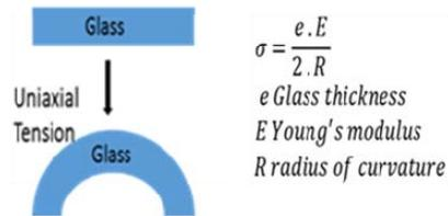
Figure 13. Bent Glass and the resulted stress
