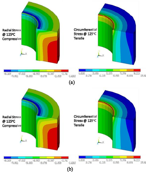
Figure 15. Stresses at (a) cold and (b) hot extremes during thermal cycling
