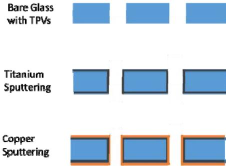
Figure 3. Glass panel fabrication process flow
