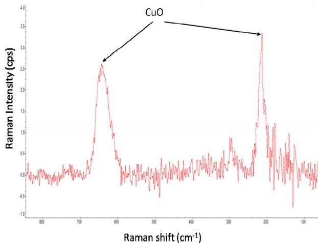
Figure 8. Raman spectrum of Copper Oxide
