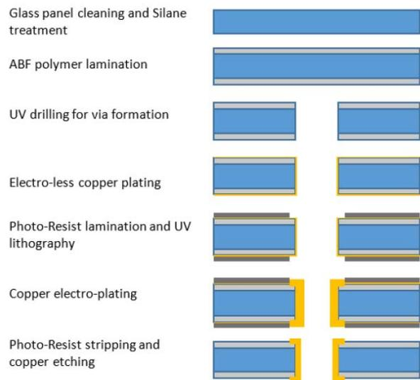
Figure 6. Fabrication process for polymer laminated glass
