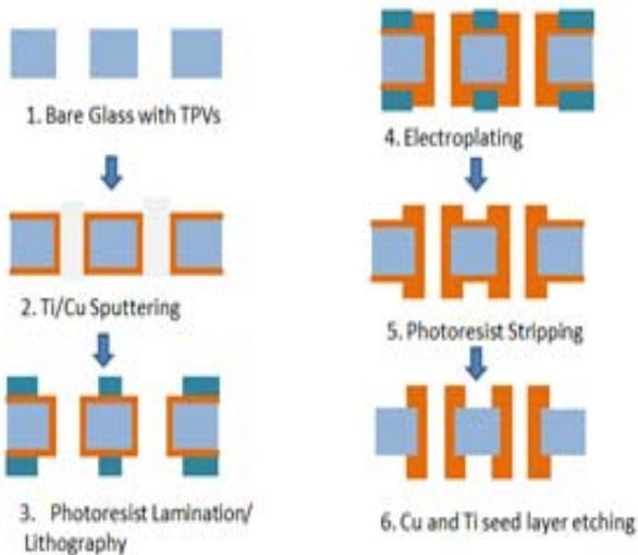
Figure 4. Glass panel fabrication process flow
