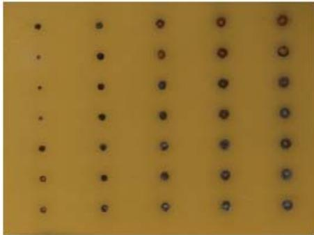
Figure 7. A glass interposer test coupon containing TPVs with different diameters
