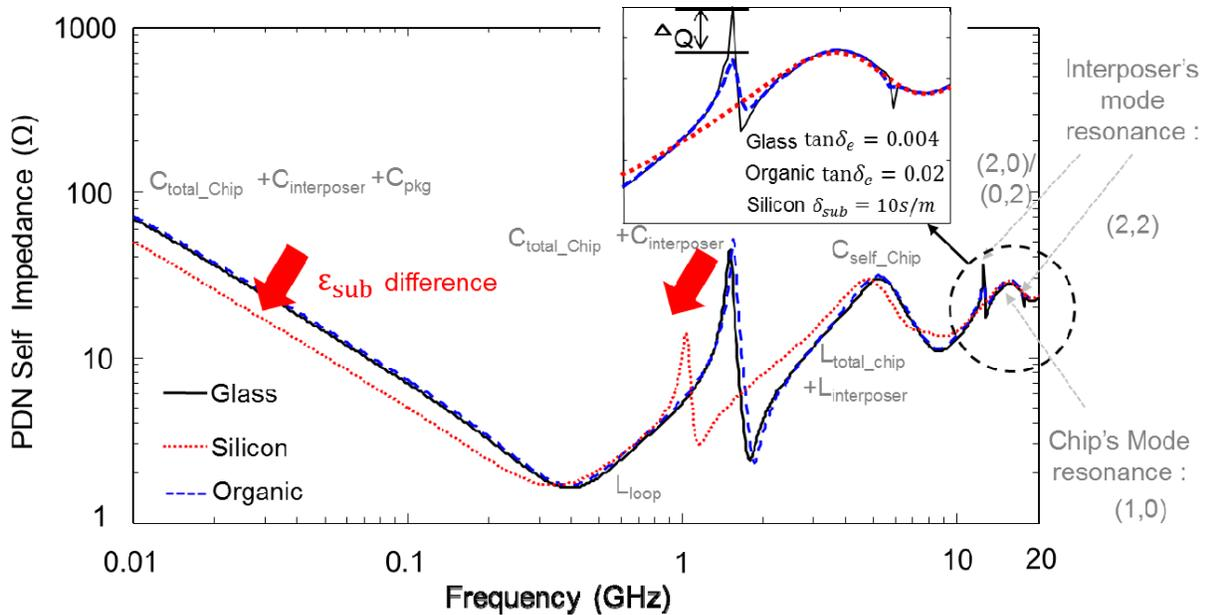
**Figure 5.** Impedance properties are simulated for the structure shown in figure 4. Depending on the interposer substrate material, hierarchical PDN impedance show different impedance profile.
