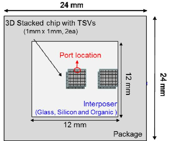
**Figure 4.** Top view and lateral dimensions of 2.5D IC to simulate and analyze hierarchical PDN impedance is shown.
