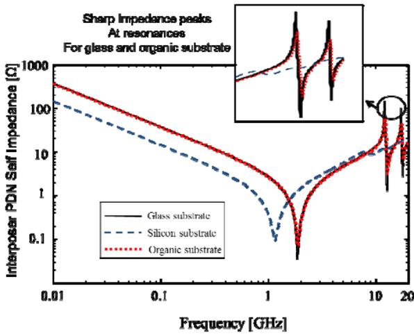
**Figure 3.** PDN Self-impedance seen at the center of glass, silicon and organic interposers are shown. Interposer PDN size is 12 mm by 12mm for all cases.
