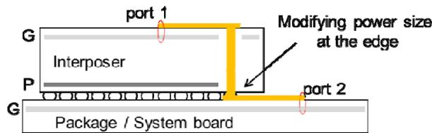
**Figure 7.** Modification of power plane to control interposer PDN cavity size
