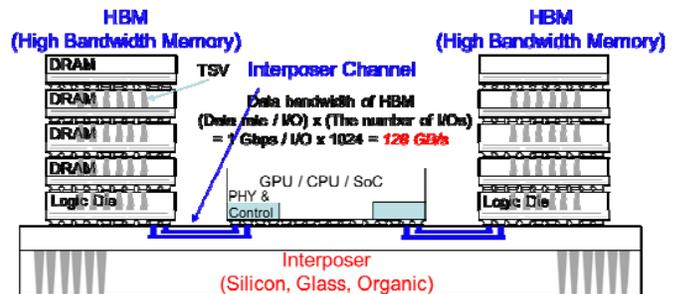
Figure 1. Cross-sectional View of 2.5D HBM module
