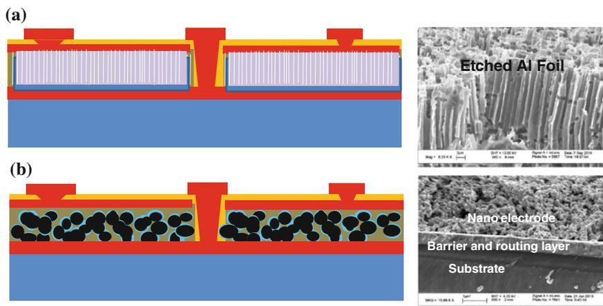
**Fig. 4** Two approaches for integrating high-density nanocapacitors in 3D IPDs. **a** Etch foil. **b** Nanoparticle electrode
