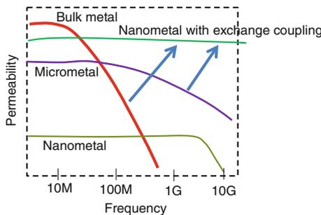
**Fig. 3** Nanomagnetic composite structure and its benefits
