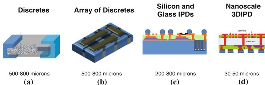
**Fig. 1** Evolution of passive components from discretely to integrated passive devices (IPDs) and 3D IPDs
