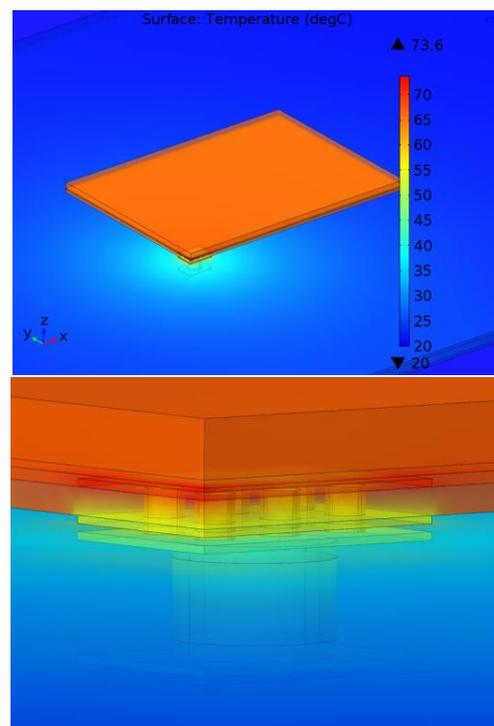
**Fig. 4.** An example of simulation result with hotspot at the die corner using an SOI PA die.
