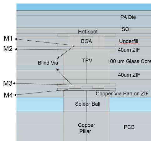
Fig. 2. Detailed structure for the modeling setup with COMSOL.
