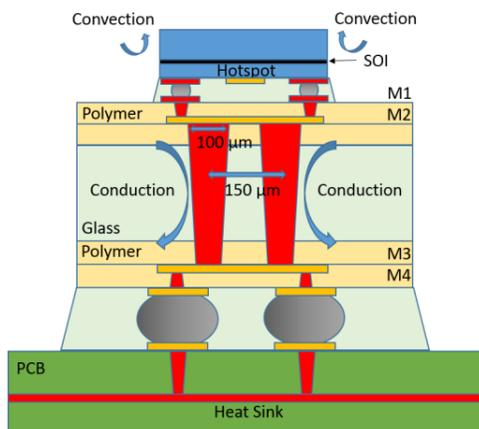
Fig. 1. RF PA Module with thermal via structures for effective heat dissipation.
