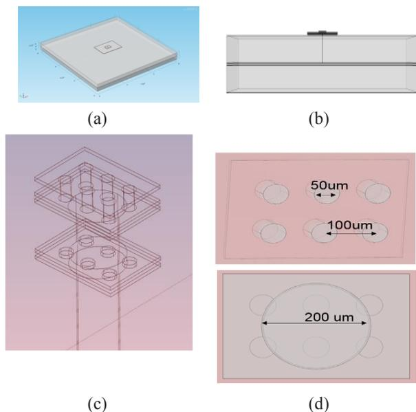
**Fig. 3.** COMSOL model construction: (a) Overall View, (b) Side View, (c) Inner View, (d) Diameter and pitch for Blind Via, and TPV.
