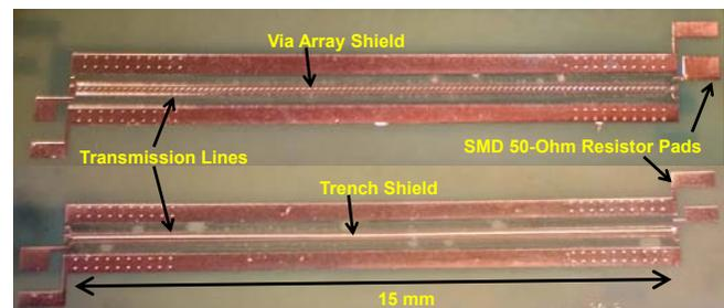
**Figure 9.** Transmission lines with Via-array and trench shield, fabricated on ultra-thin glass substrate.
