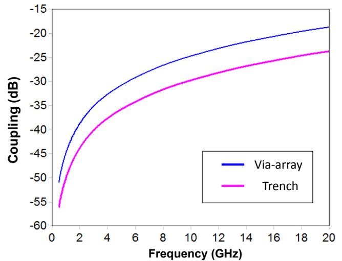
**Figure 8.** Comparison of TL-TL coupling in presence of via-arrays and trenches.
