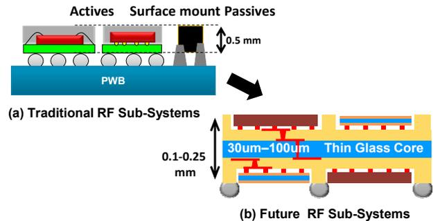
Figure 1. The new 3D IPAC approach for RF modules vs. traditional.
