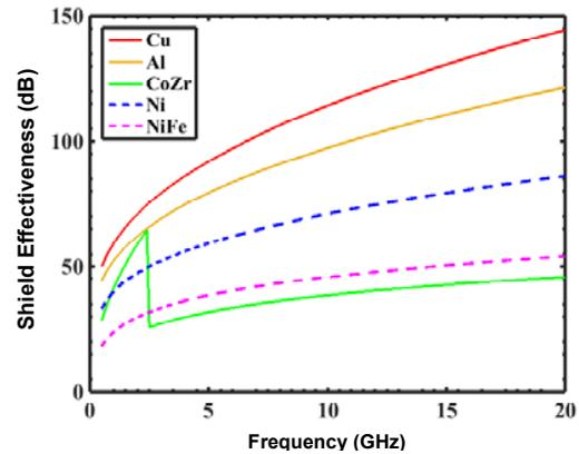
Figure 5. Comparison of shielding effectiveness of different materials.
