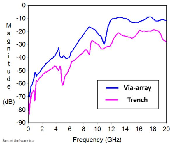
**Figure 10.** Comparison of measured TL-TL coupling in presence of via-arrays and trenches.
