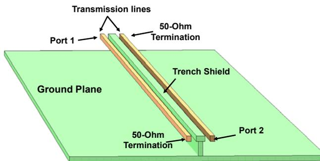
**Figure 7.** Simulation set-up showing transmission lines separated by a trench-based shield.
