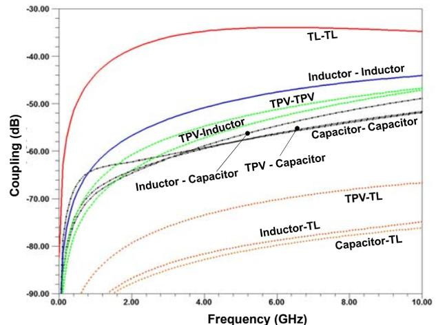
Figure 4. EM coupling between package elements.
