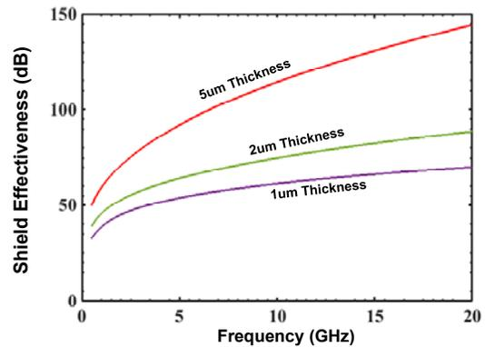
Figure 6. Shield effectiveness with varying thickness of the shield metal.
