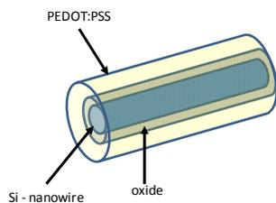
Fig. 2: Schematic representation of an individual nanowire capacitor.
