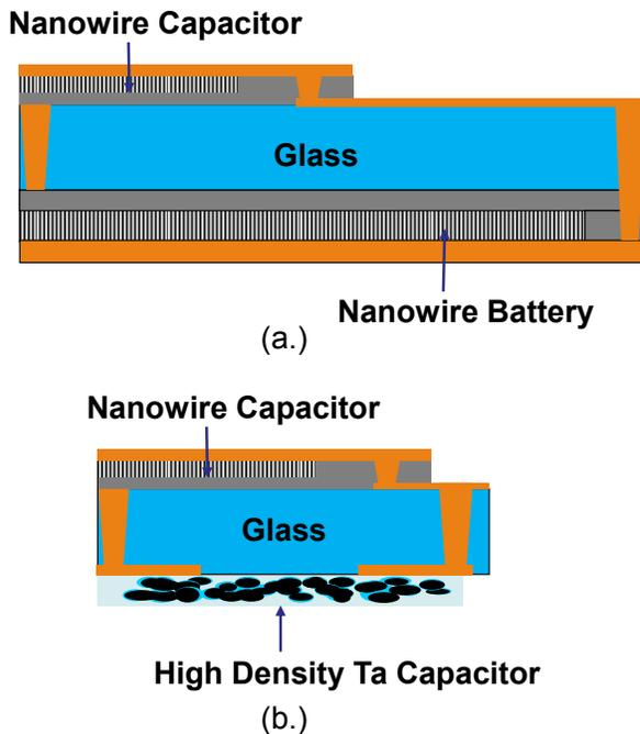
Fig. 1: Different configurations of Si-nanowire capacitors as 3D IPDs (a.) with Nanowire batteries to form self-sustained sub-system and (b.) with high density Ta capacitor to form a heterogeneous VRM+decoupling solution.
