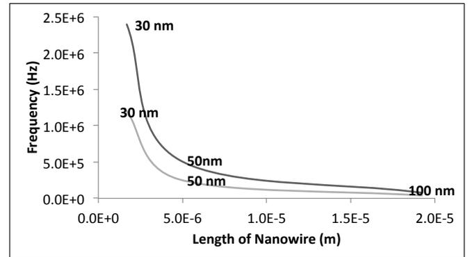
Fig. 4: Change in cut-off frequency with increasing nanowire length. It is important to note that the length of the nanowire changes based on the size of the Au catalyst.
