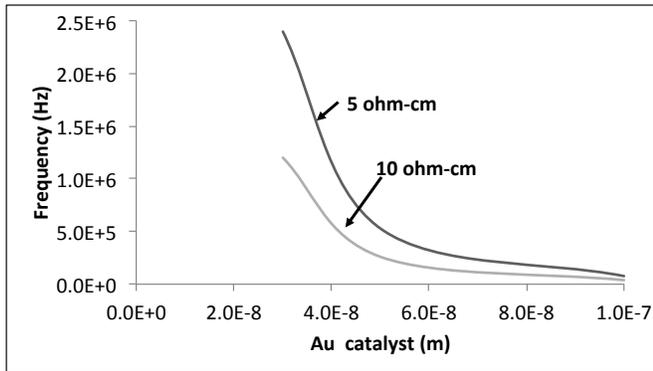
Fig. 5: Change in cut-off frequency with respect to Au catalyst size.
