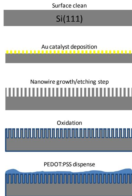
Fig. 6: Fabrication process for capacitor formation starting from surface preparation to top-electrode formation.
