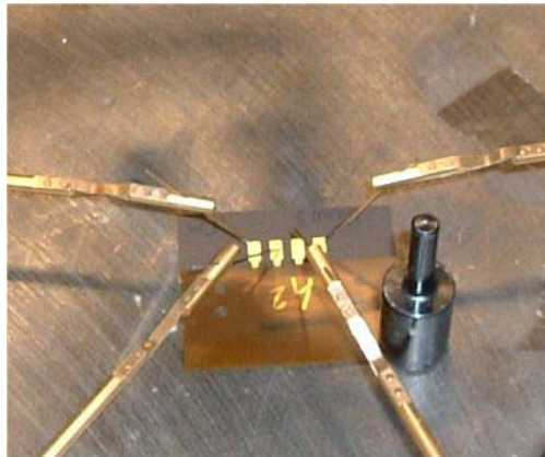
(fig 4) Closer look at Four-Point Probe test
